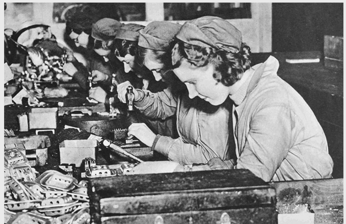
Producing component parts for the Spitfire at the Supermarine works at Southampton : Girls drilling and punching holes in metal accessories.
